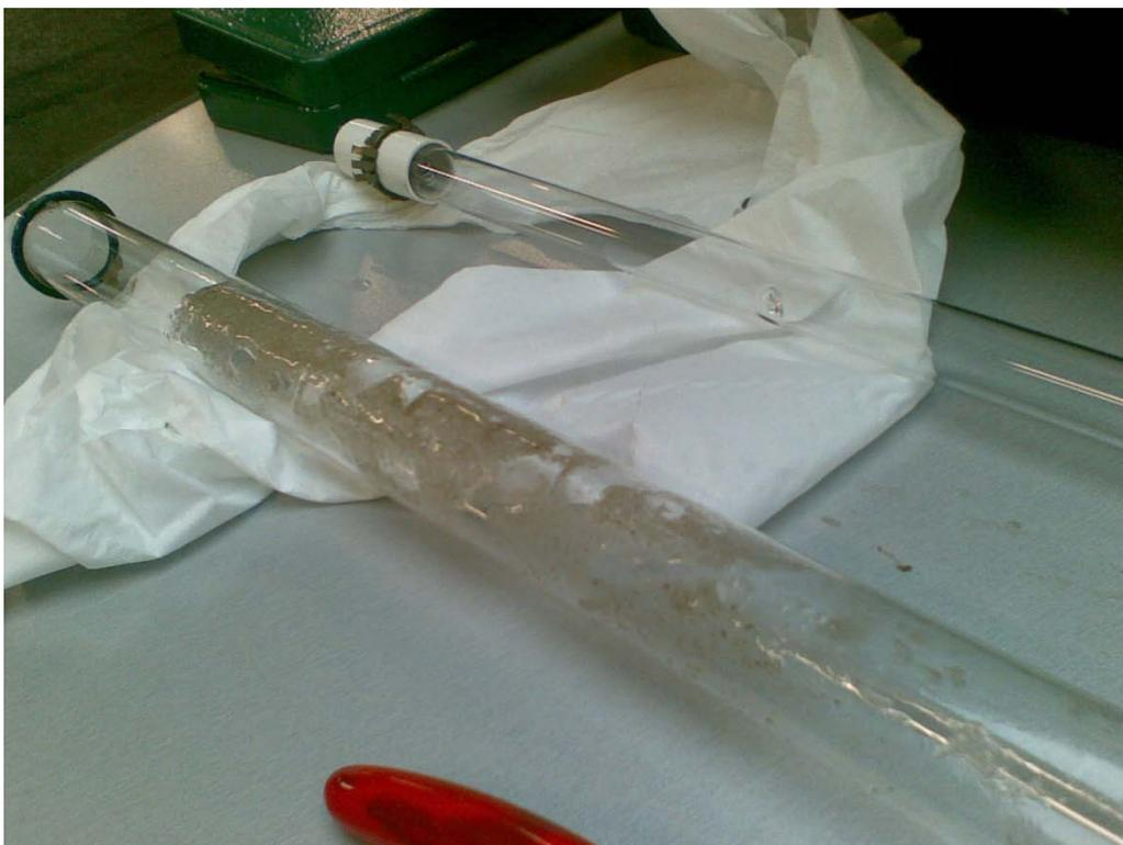
After 24 hours: totally cleaned quartz sleeve and UV reactor
