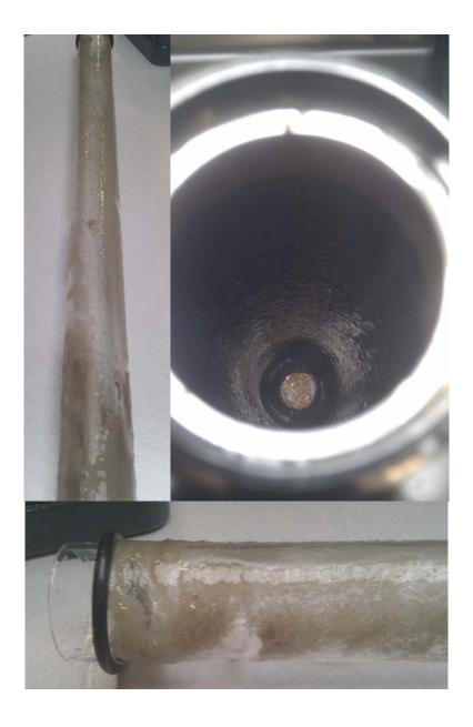
The biofilm is formed on the quartz sleeve but also in the reactor (bound to the metal)
